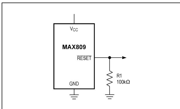
Figure 2.  $\overline{\text{RESET}}$  Valid to  $V_{CC} = \text{Ground}$  Circuit
