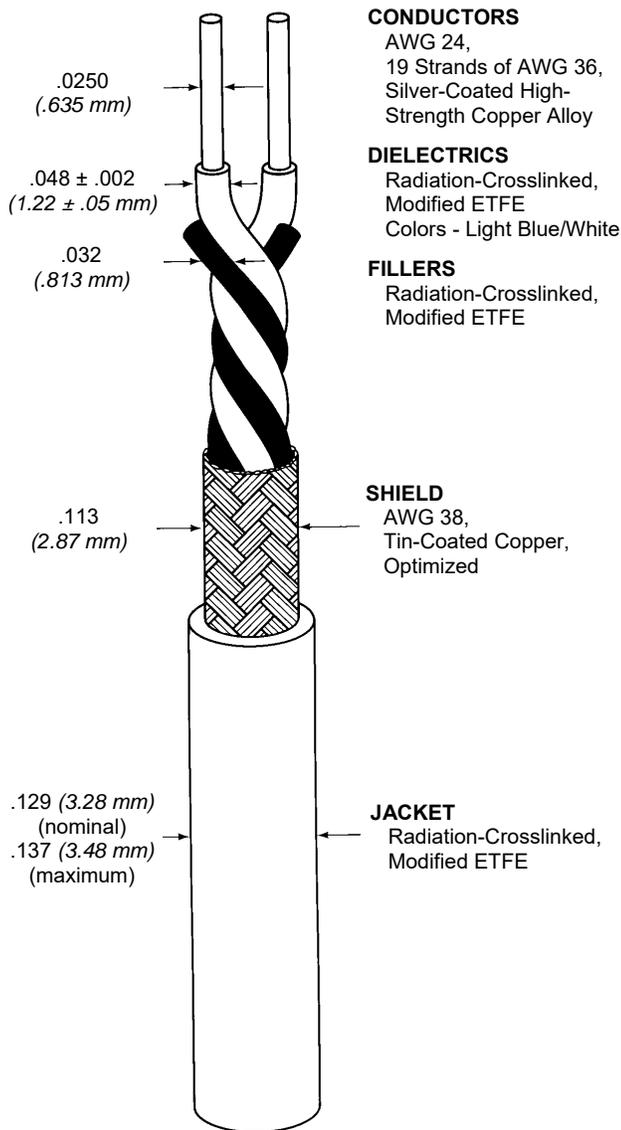
The conductor AWG size and outer jacket color will be appended to the part number. Unless otherwise specified, outer jacket color will be white designated by a "-9" in accordance with MIL-STD-681, (e.g. 10612-24-9).
